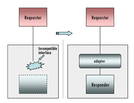
Figure 3 - Adaptor pattern diagram
